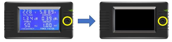
Always press gently on the button positioned to the right of the display, pressing with force can potentially damage the meter.
